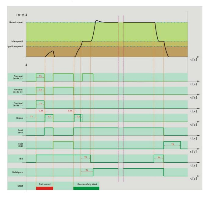
T1 – start delay T4 – safety-on delay T2 – crank time T5 – idle time T3 – pre-heat time T6 – Stop delay
