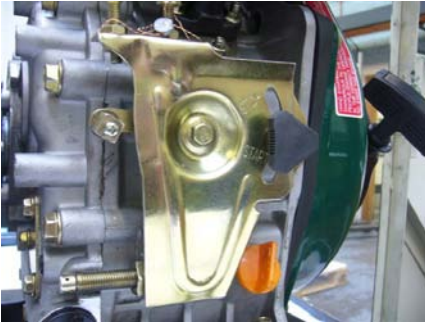
Figure 5.2.3 Engine Control - Variable Speed
