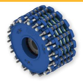
The WPT Power fail-safe disc brakes are springapplied and air released. The Pin Drive Low Inertia style is commonly used for applications requiring high-energy high-torque stopping power, and parking. These are well suited for a wide variety of applications including those where high cyclic and high inertia stops need to be absorbed and dissipated easily.
